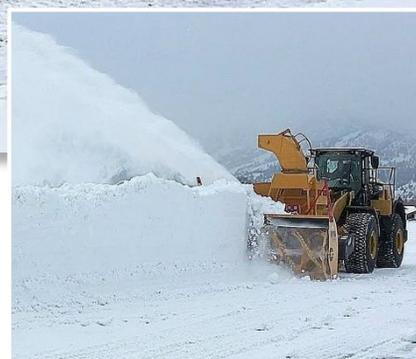
RPM48R featuring the optional truck loading chute.
