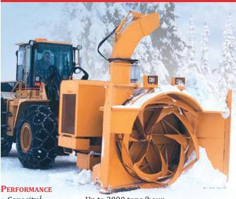
Capacity<sup>1</sup>: Up to 3000 tons/hour
