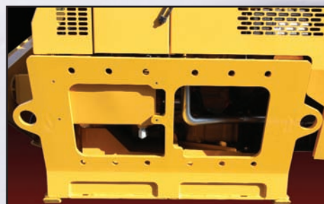
Quick attach plate receiver with optional welded or bolted.
