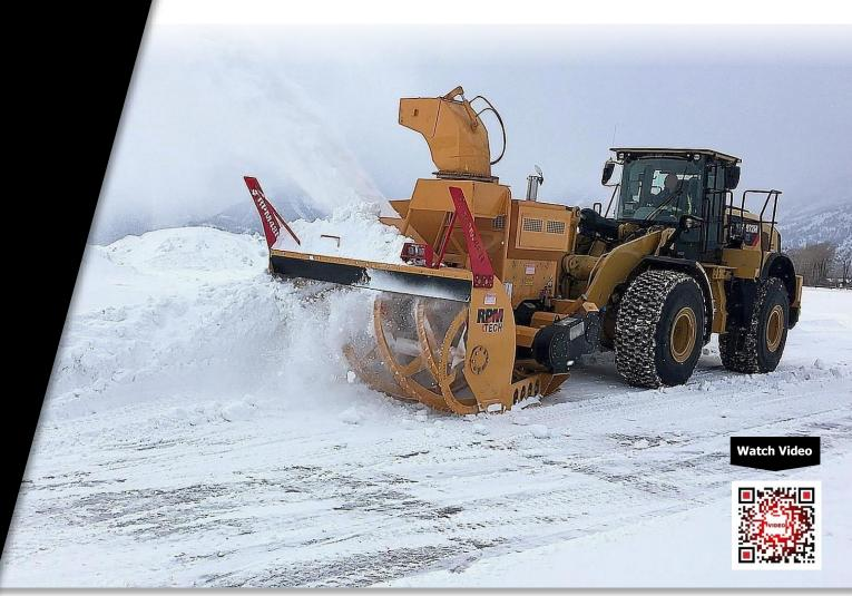
RPM48R featuring the optional truck loading chute.
