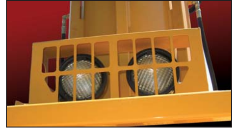
Two optional work lights can be installed on top of the snow blower body to improve visibility during snow removal operations.
