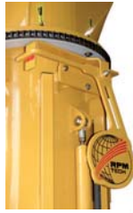
The pendulum installed on the chute indicates whether the snow blower is level.
