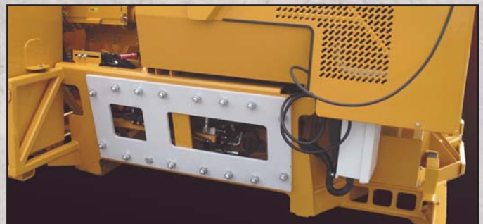
The electrical box is sealed, and the hydraulic system for the valves and controls is protected from debris.
