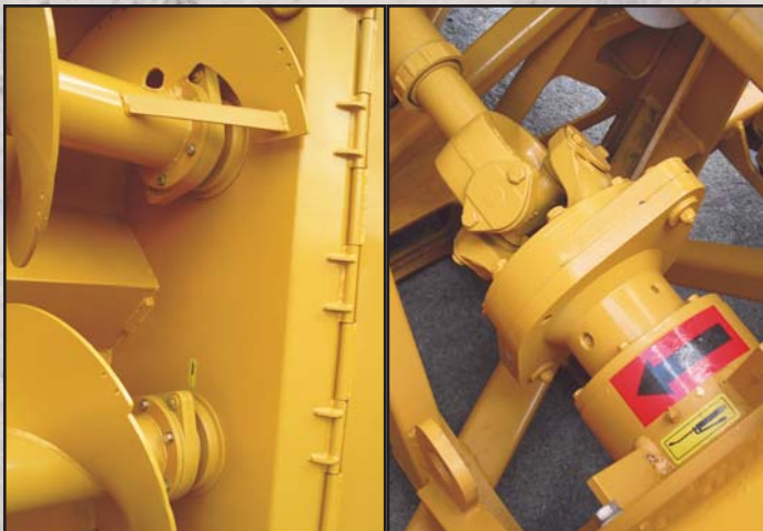
Three sets of shear bolts protect the impeller and the augers: one set located on the drive shaft and two sets located on the front augers.
